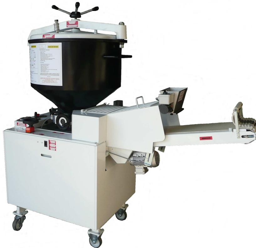
The closed hopper divider is designed to divide the dough in equal weight. It distinguishes itself of a hydraulic divider by the fact that the whole dough in the fork kneader bowl can be spilled in one time via a bowl lift in the exit of the fork kneader. Besides, it has a belt allowing to provide an automatic intermediate proofer or to take back manually the dough.
