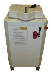
The hydraulic divider DL20C is designed to divide the dough in equal weight. The square divider allows getting some square pieces of dough for a direct making of "paved" Thanks to their studies shapes, they allowed a completely uniform spreading out of dough on the whole surface and the covers.
