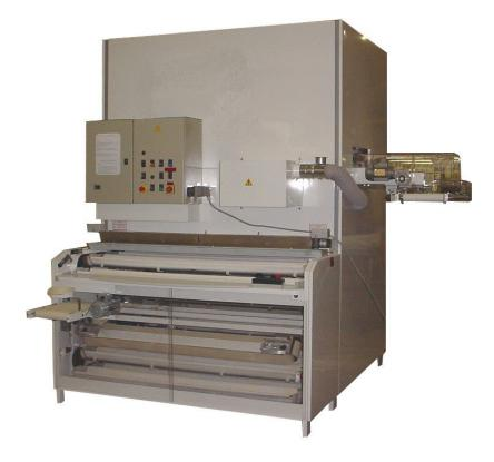
The mixed intermediate proofer allows charging by hand as well as automatically. They can be used for the white breads of for special breads.
