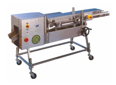
The side cut belt driven is intend to cut entirely or partially in the lengthwise products as baguettes, small breads, croissants, donuts, eclairs, hot-dogs, hamburgers...
