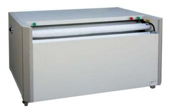
The purpose of the intermediate proofer is to allow for the resting of the bread dough once it has been divided, to develop the flavors and taste of the breads and at the same time facilitate the moulding process.
