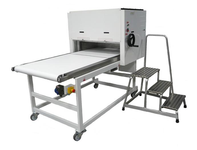
The dough processing and weighing table allows for effortless and consistent chuncking of dough out of the mixer. It functions in conjuction with a lift/tiltable mixer or bowl lift. The main advantage of this equipment is that the operator works at table height and will not suffer from any effort to cut dough pieces out of the mixer and carrying them on a work table.
