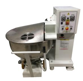
The fork kneaders with removable bowl allow the transfer of the dough more easily until the bowl lifter thanks to their integrated transport trolley of the bowl. Besides, it facilitates the resting of the dough.
