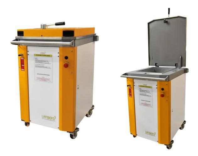
The DL20 KAF square dough divider is designed to divide dough into 20 equal-weight pieces. Thanks to its special shape, the dough is evenly distributed over the entire surface of the bowl. The flour anti-splash kit complies with hygiene standards and conformity of use requirements.
